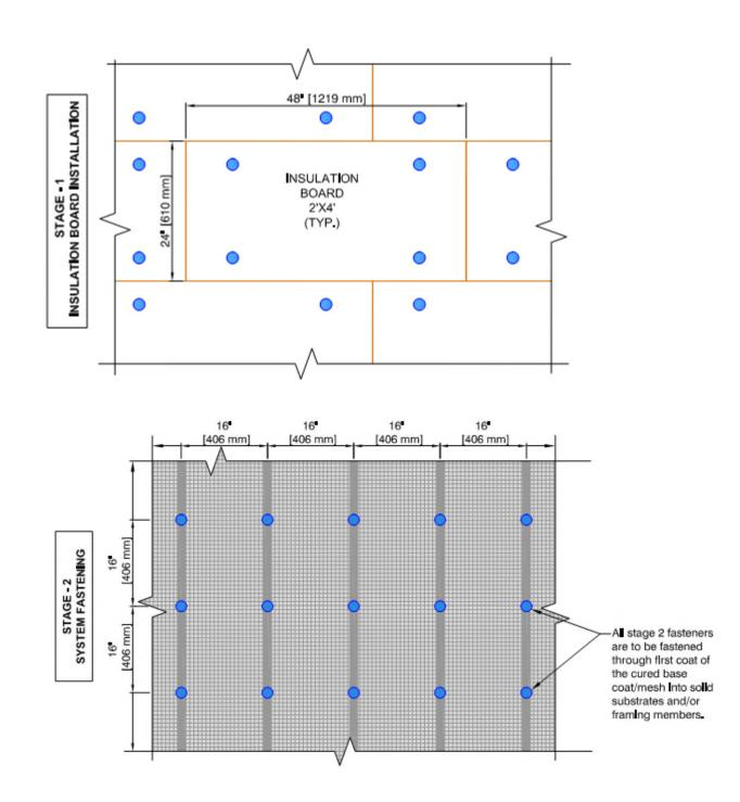
*SPEC NOTE:* The above fastening pattern addresses recommended fastener placement for typical wall installations.
